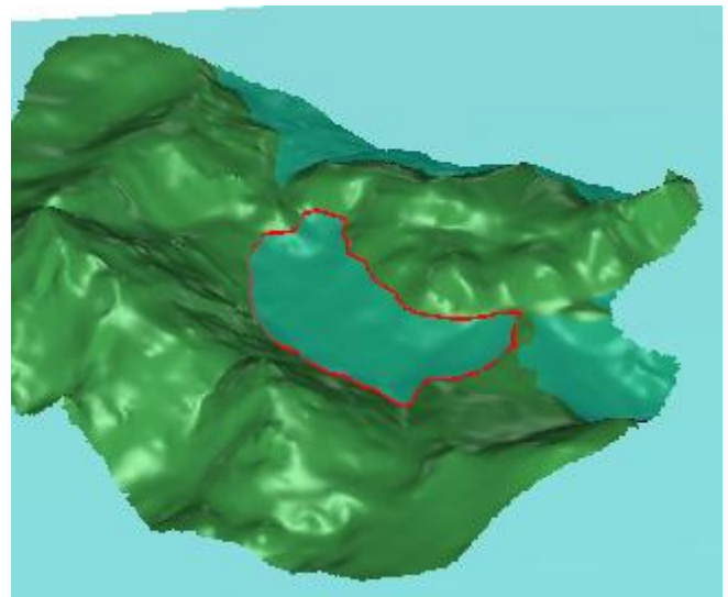
Figure 4: Using the command intersection to calculate the contour of the lake
